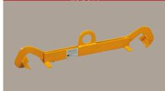
"Note: Drum lifting clamps must only be used with drums that have lids attached. W.L.L. 500 kg. AS4991-2004 Will lift one 205 litre drum with forklift or engine crane. Carton Dimensions L76cm x W11cm x H15cm Weight 5kg"
